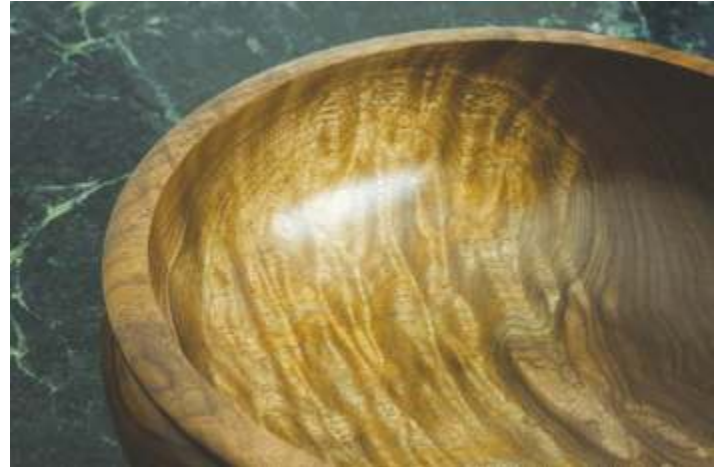
Five coats of an oil/varnish blend and a surface film has begun to build a semi-gloss surface on this quilted-walnut bowl.
