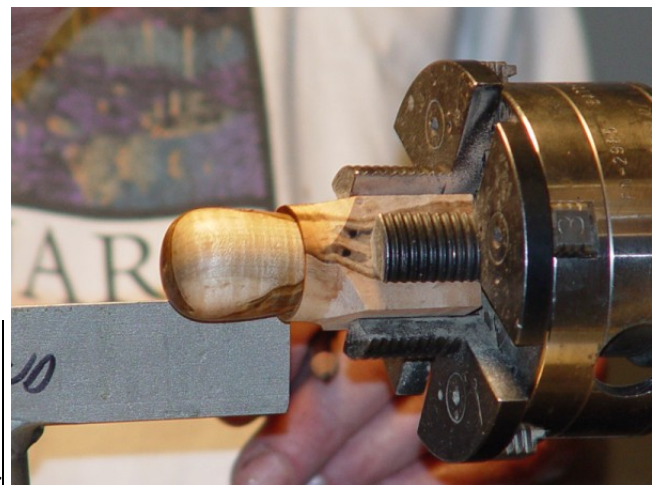
Reverse turning the birdhouse on a jam chuck
