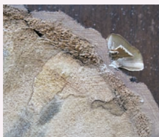
Mushrooms on the outside often directly correlate to where the spaltting is occurring on the inside.
