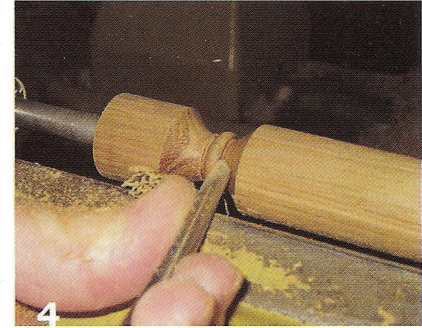
4 Complete most of the detail work with a 3/8" or 1/2" spindle gouge.
