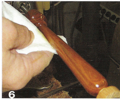
6 Apply a penetrating oil with paper towels. (Cloth rags present a safety hazard.)
