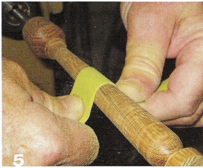
5 Sand the handle with 150 grit, then 180 grit and finish up with 220 grit.
