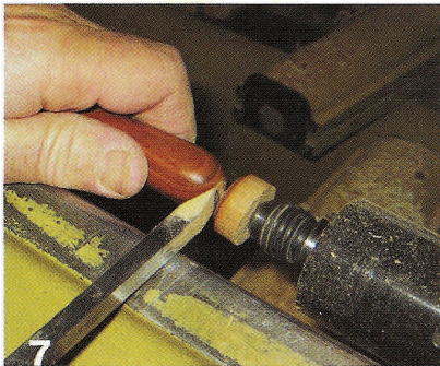
7 With a skew, separate the waste from the tailstock end.
