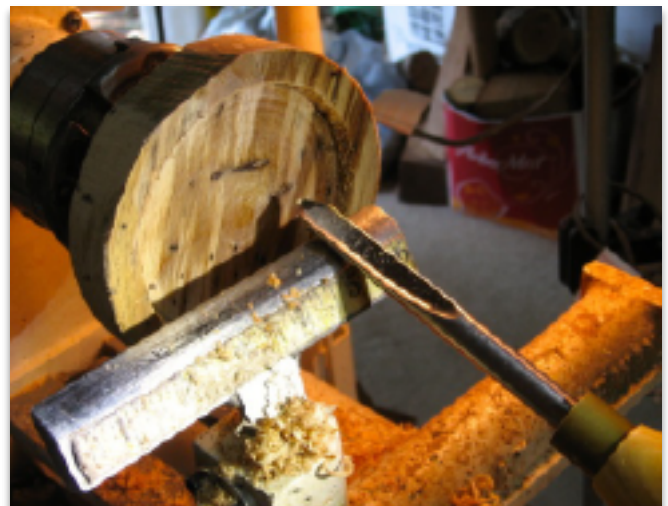
Preparing the 4" Recess for the Mirror
