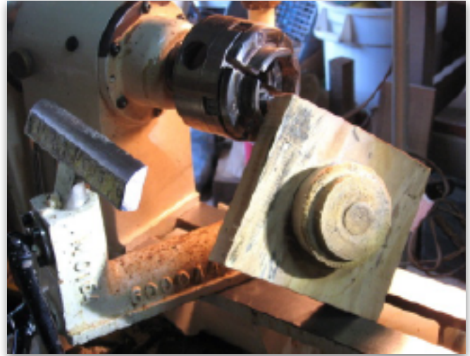
Mirror Blank with a Glue Chuck
