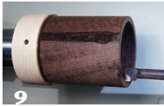
9 After drilling out the bulk of the outer wood, use a boring bar to match the dimension of the inner assembly. Note the small hole drilled through to allow air to escape when the pieces are assembled.
