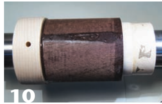
10 Only apply glue on the bottom inside of the outer wood, then assemble and clamp in the lathe until cured.
