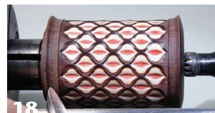
18 On your regular lathe, turn a profile on the base and lid of the box while the lid is held in place securely with the tailstock.
