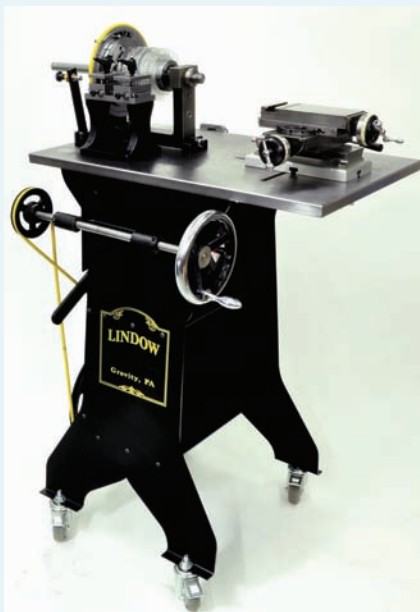
Lindow Rose Engine with sliderest, 2007. For more, visit roseengineturning.biz .
