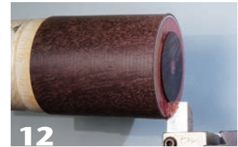
12 Trim the excess off the end of the assembly, showing the thin layers around the inner core of pink ivory.
