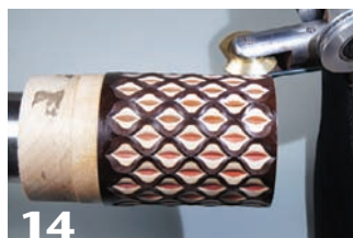
14 Cut the pattern with multiple passes, each going a bit deeper. Soak with CA glue after each pass.
