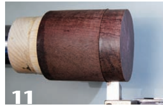
11 After parting off, turn the exterior, leaving a very thin layer of the outer Katalox wood.
