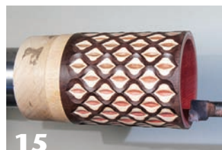
15 Drill out the bulk of the inside of the box, then use a boring bar to cut to the final dimension.
