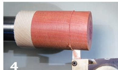
4 Make multiple cuts to reduce the outer diameter of the core.
