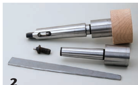
2 An MT2 to MT3 adapter sleeve can be used if necessary, but may require inserting a screw into the end of the arbor to permit removing the sleeve with a tapered knockout bar.
