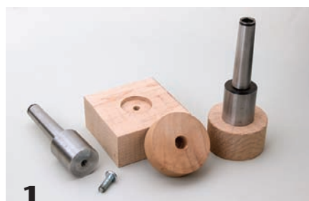
1 Drill and tap a blank Morse taper arbor for a screw. Mount a scrap wood block onto the arbor.
