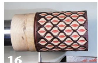
16 Part off with the cut-off tool and catch the cylinder on your finger.
