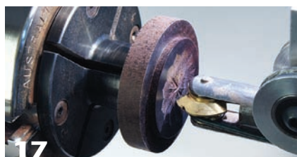
17 The base of the box has a tenon cut to match the inside of the cylinder and can be decorated with the rose engine.
