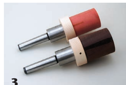
3 The inner core of pink ivory and the outer layer of Katalox are mounted on MT2 arbors to enable moving from one lathe to another. Note the vent hole in the waste block on the lower piece.
