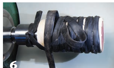
6 Glue the veneer onto the core cylinder and wrap with rubber bands (long strips cut from an inner tube work well).
