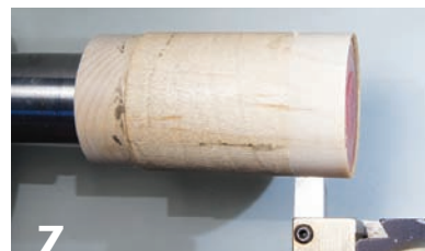
7 When dry, soak with CA, give it a shot of accelerator, then trim down, leaving a very thin layer of the maple veneer.
